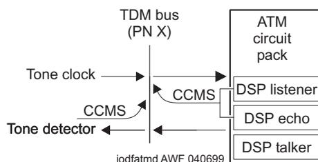
Figure 9-8. ATM Board DSP Test (#1293)
