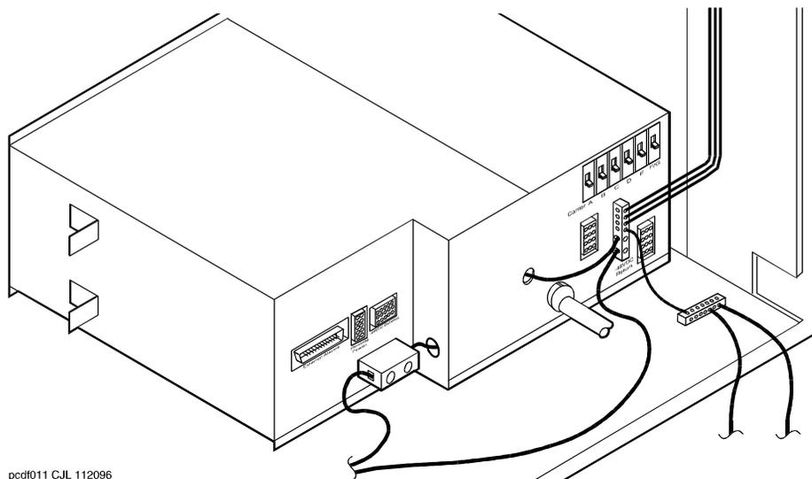
Figure 9-19. Power Distribution Unit (J58890CH-1)
