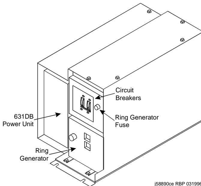
**Figure 9-15. AC Power Distribution Unit (J58890CE-2) — Front**
