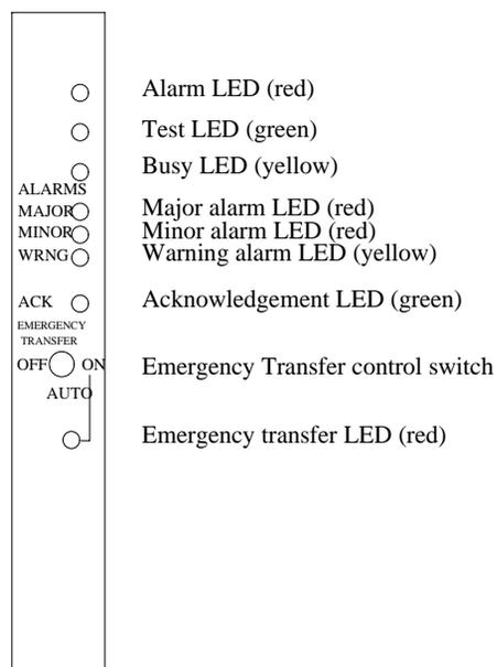
Figure 7-1. SYSAM and EPN Maintenance Circuit Pack LEDs
