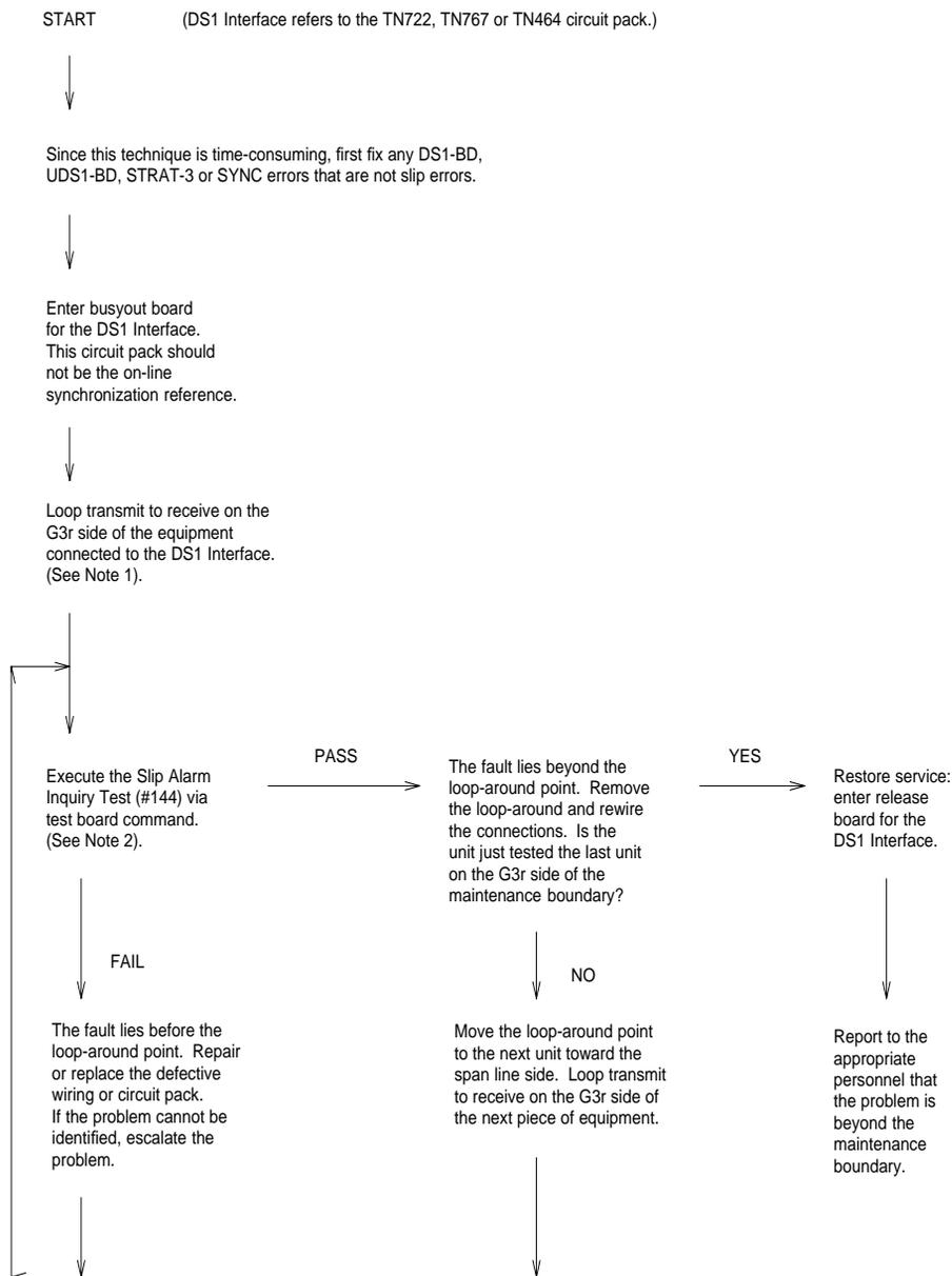
Figure 9-104. Facility Fault Sectionalization
