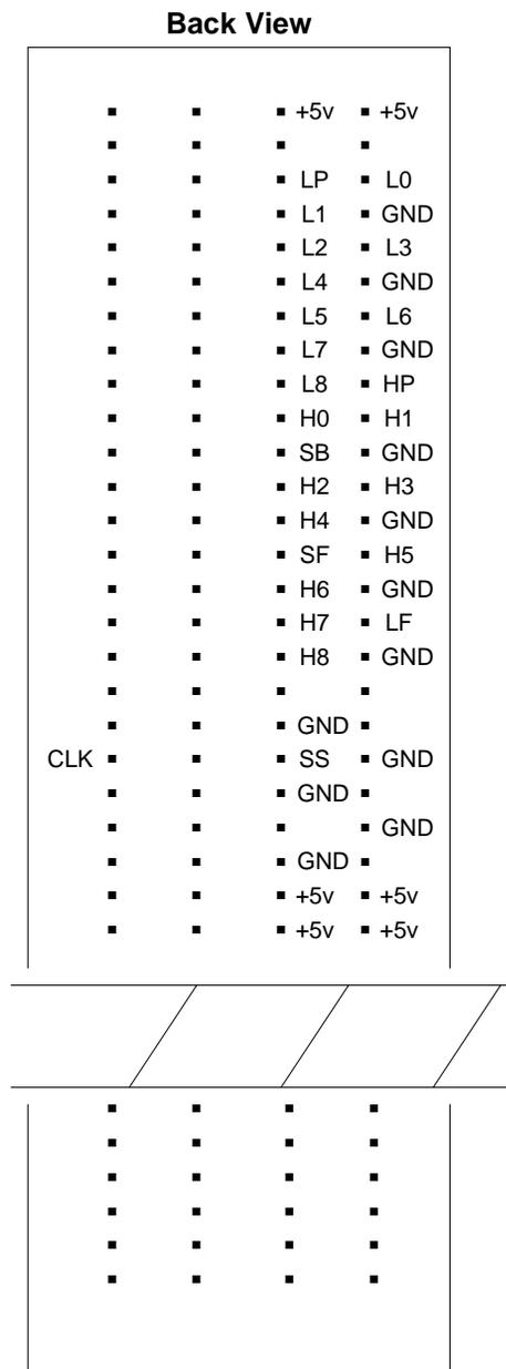
Figure 5-44. Packet Bus Leads on the Backplane
