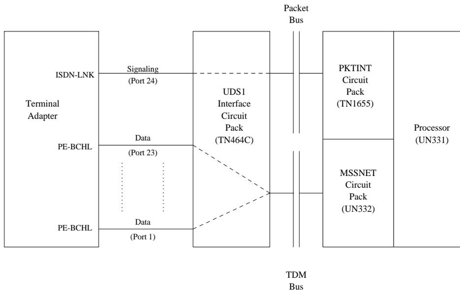
Figure 9-72. PRI Endpoint Port Interactions
