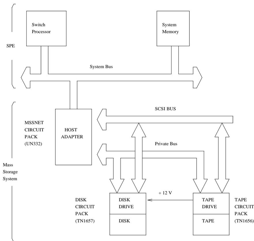
Figure 9-23. Mass Storage System Interactions
