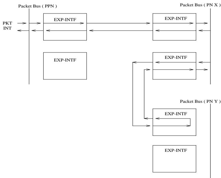
**Figure 9-48. Expansion Interface Packet Interface Test-EPN to EPN link**
