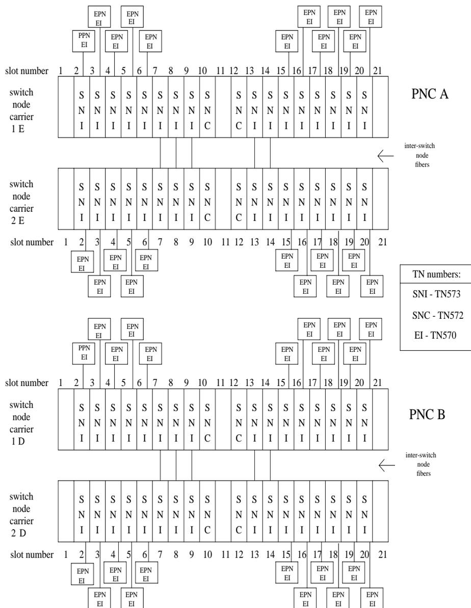
Figure 9-88. CSS Configuration with Duplicated PNC and 4 Switch Node Carriers
