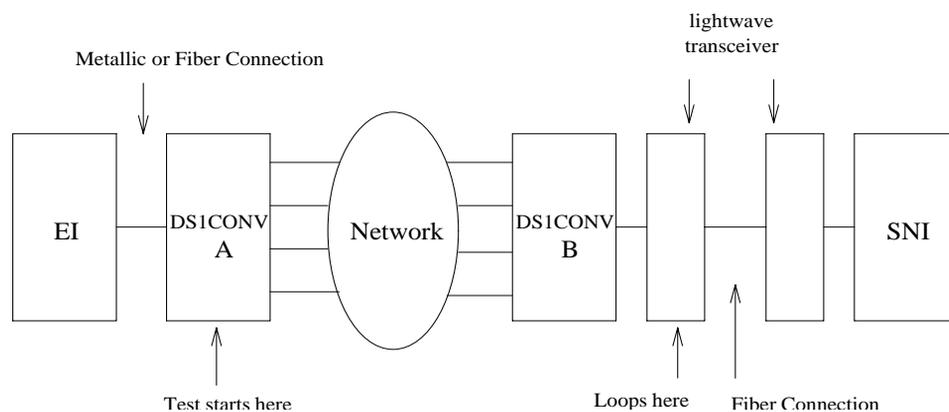
Figure 9-34. Far-end Lightwave Transceiver Loopback Test
