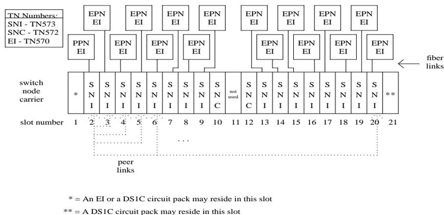
Figure 9-87. CSS Configuration with Simplex PNC and 1 Switch Node Carrier
