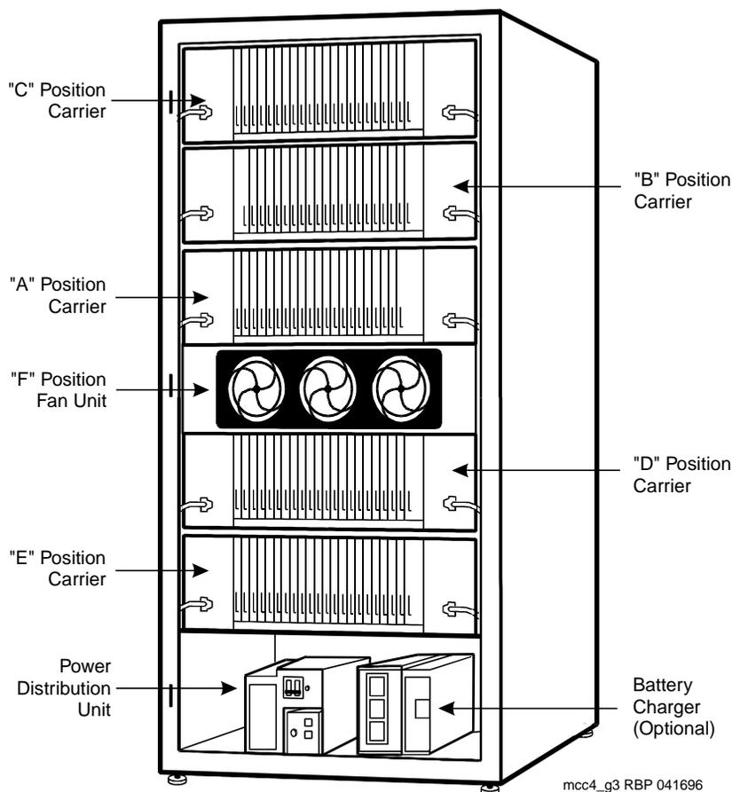
Figure 9-17. AC Power Distribution in Multi-Carrier Cabinets
