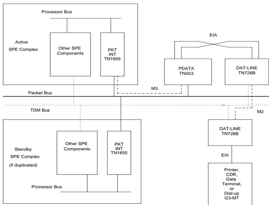
Figure 9-66. Typical System Port Connection
