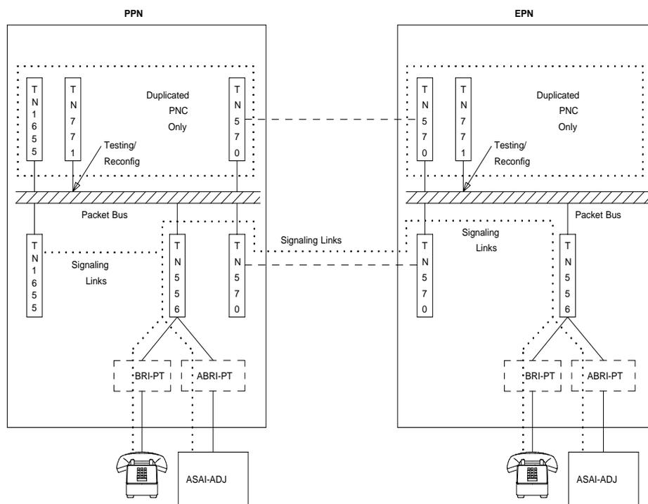
Figure 5-40. ISDN-BRI/ASAI Packet Bus Connectivity
