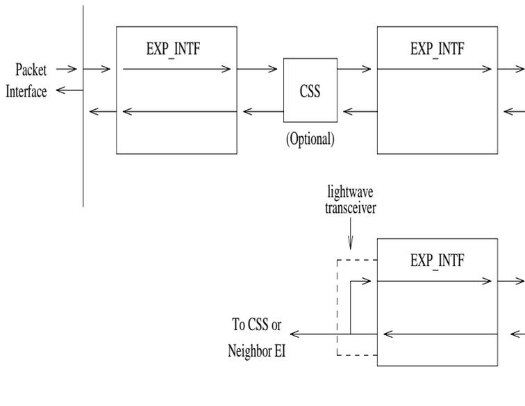
Figure 9-44. Packet BUS Lightwave Transceiver Looparound—EPN only
