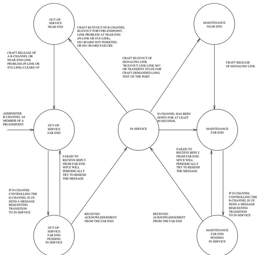
Figure 9-73. Common Progressions in PRI Endpoint Service States
