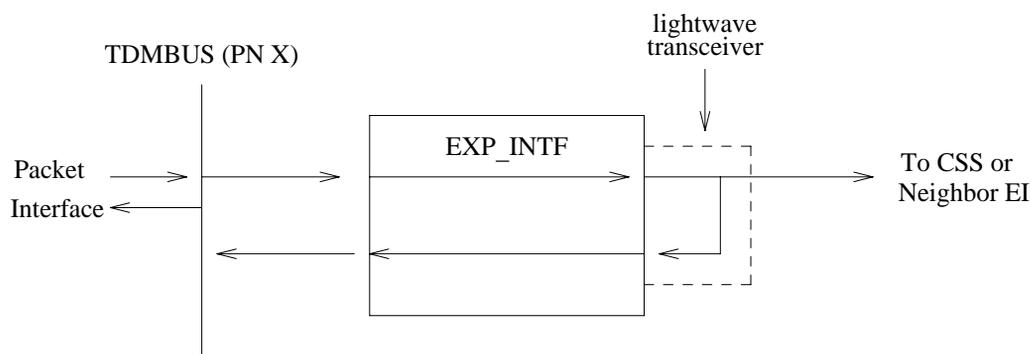
Figure 9-43. Packet BUS Lightwave Transceiver Looparound—PPN only
