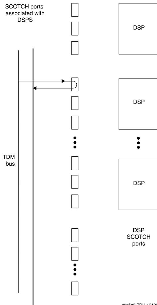
Figure 9-117. VC Circuit Pack DSP Port Local TDM Loopback Test
