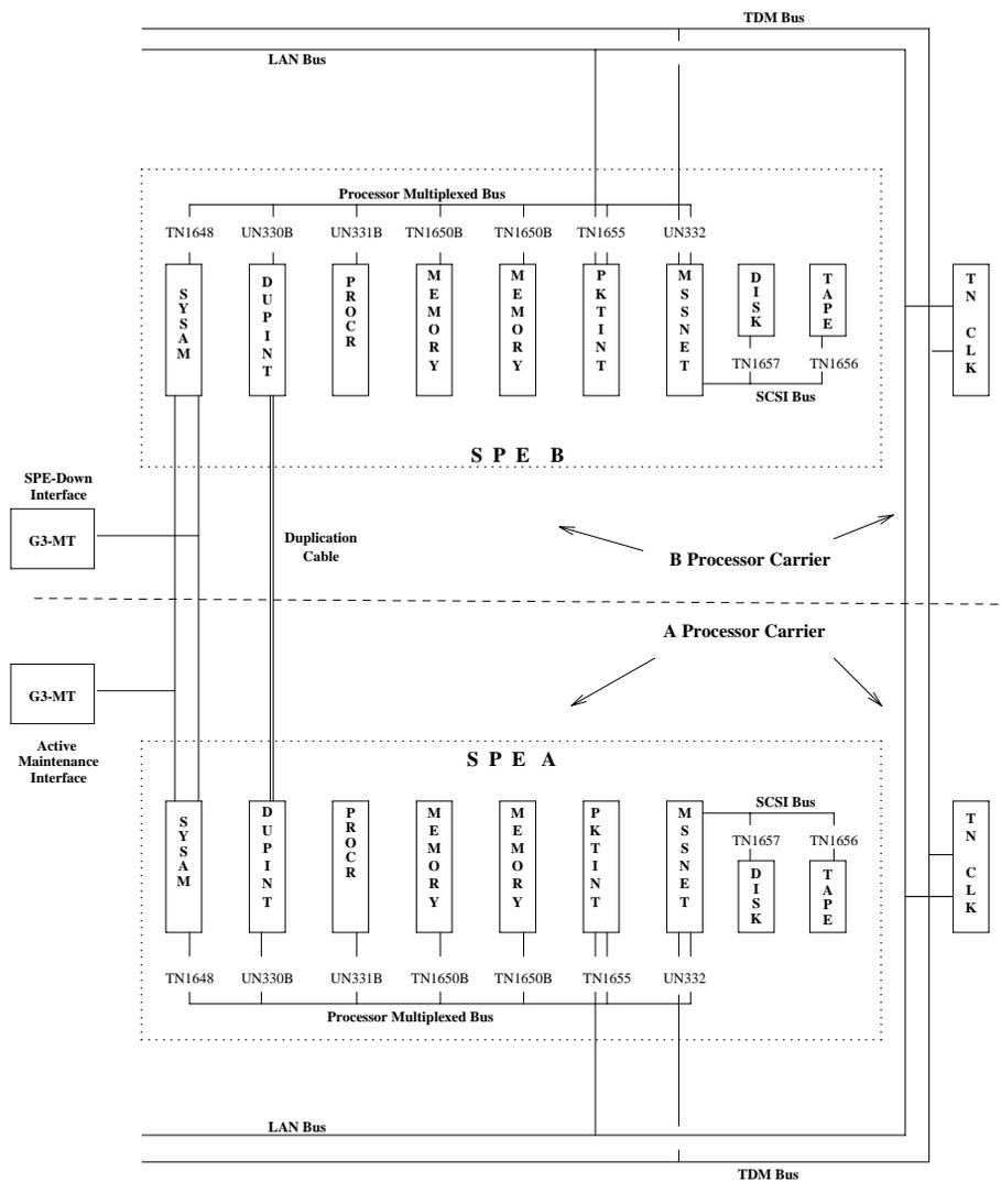
Figure 1-3. Duplicated SPEs — Hardware Configuration
