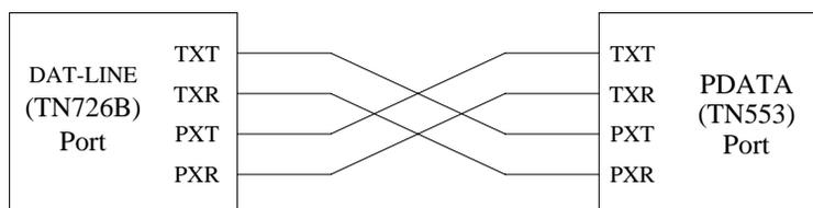
Figure 9-67. System Port Wiring Scheme
