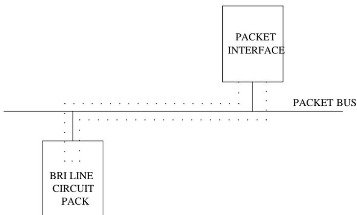
Figure 9-12. Path of the BRI Port Local LAN Loop Around
