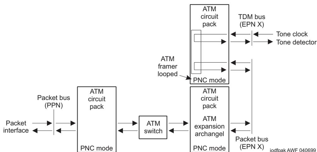
**Figure 9-6. ATM Board Framer Looparound Test (#1260)
