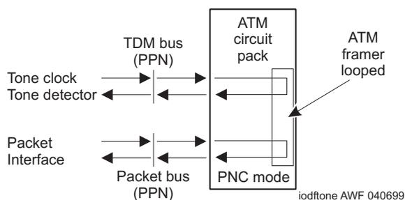
**Figure 9-5. ATM Board Framer Looparound Test (#1260)**
