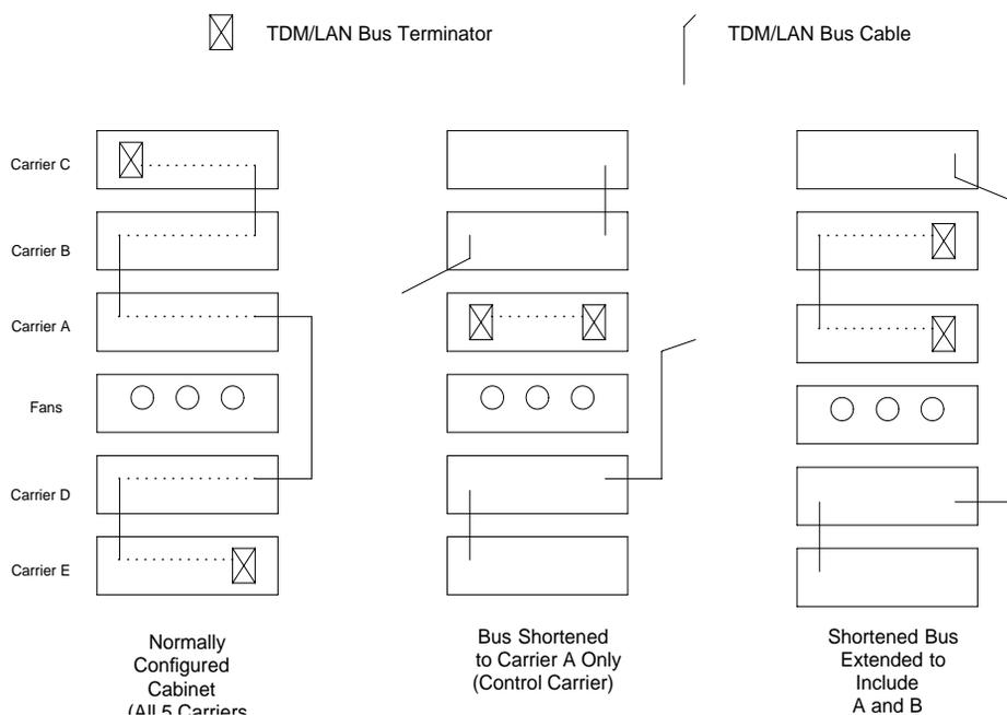
**Figure 9-110. Carrier Rewiring Example—Rear View of Five-Carrier Cabinet**
