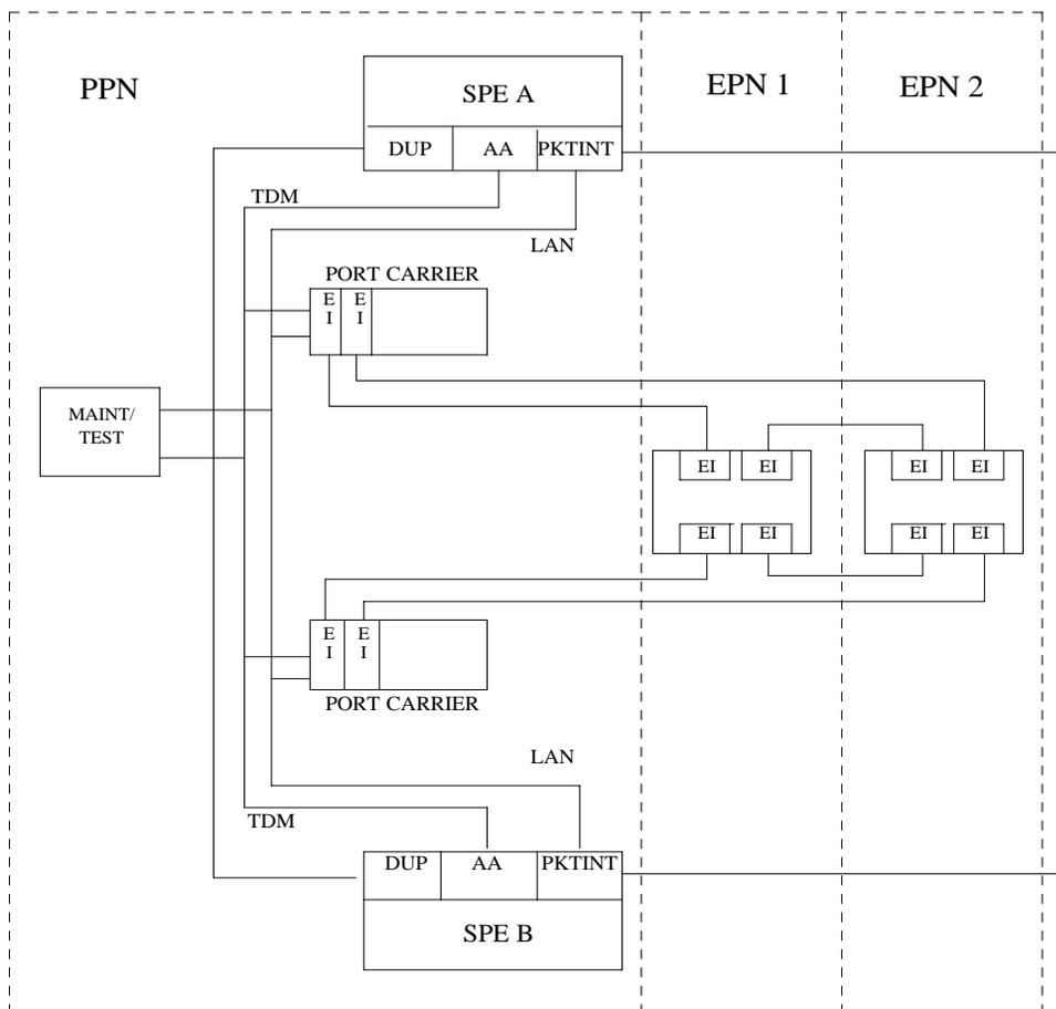
Figure 9-78. Duplicated Direct Connect PNC Connectivity
