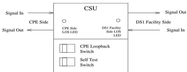
**Figure 9-27. Typical CSU Maintenance Capabilities**
