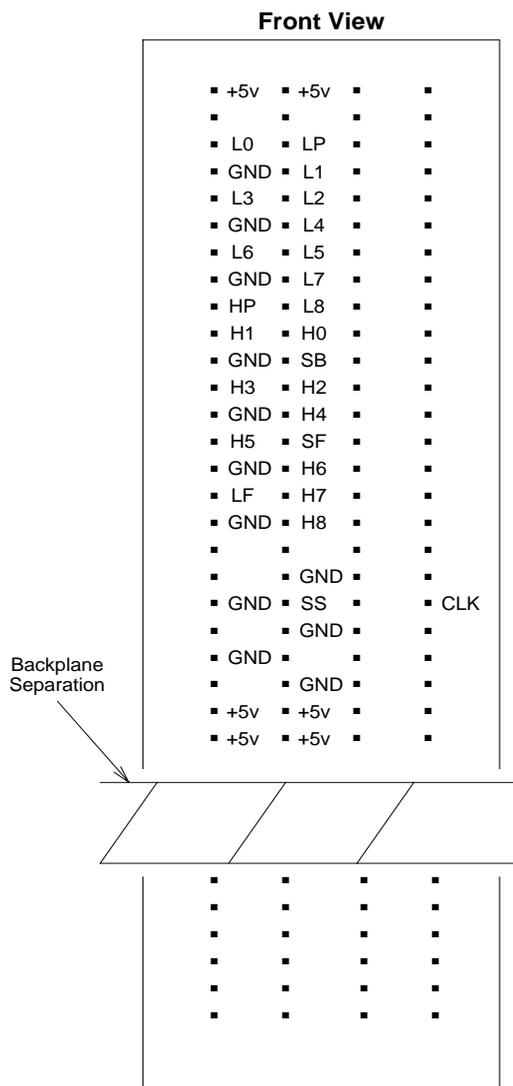
**Figure 5-43. Packet Bus Leads on the Backplane**
