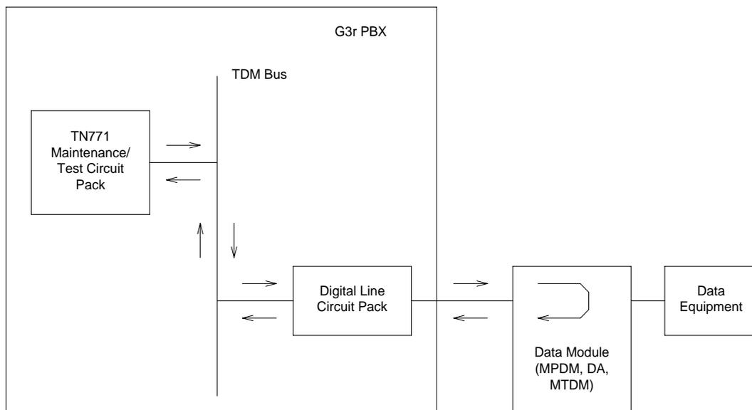
**Figure 9-71. Internal Looparound Test**
