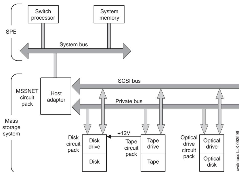
Figure 9-81. Mass Storage System interactions
