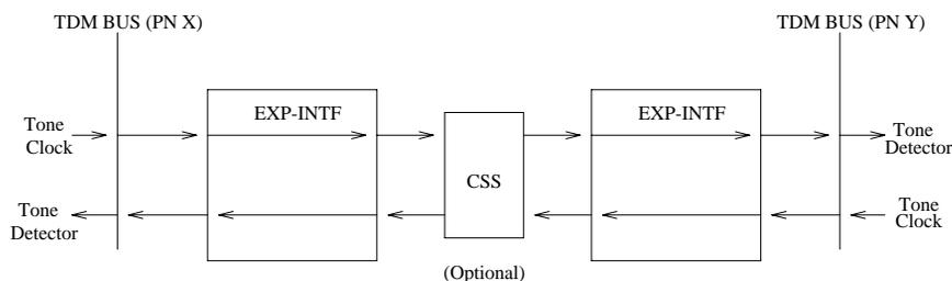
**Figure 9-41. Two-Way Circuit Switch Transmission Test**
