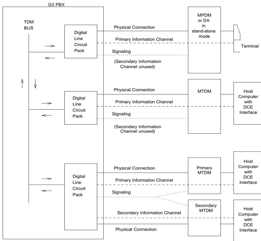
Figure 9-70. Typical Data Module Configurations
