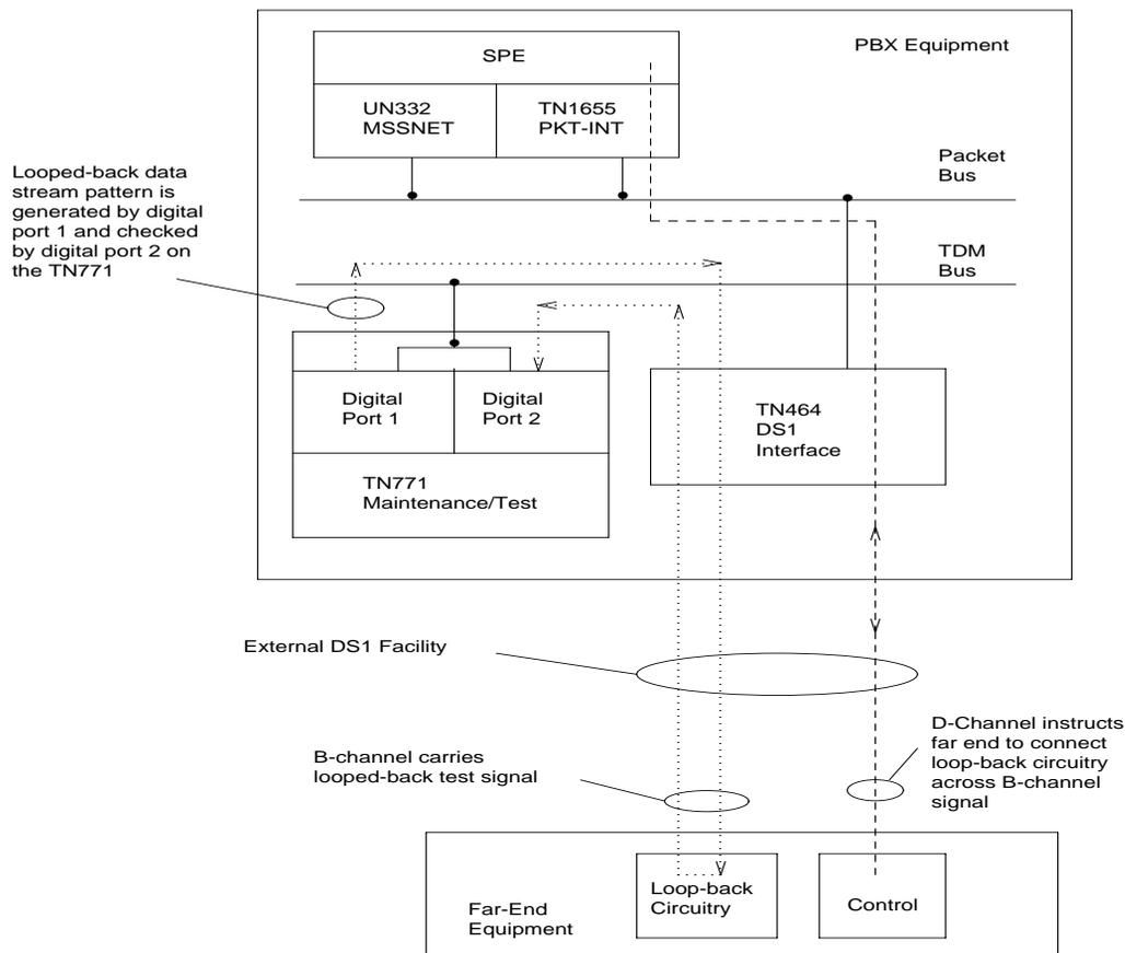
Figure 9-64. ISDN-PRI Outgoing Test Call
