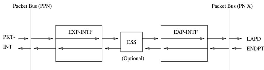
Figure 9-45. Expansion Interface Packet Interface Test—Packet Endpoint Loop
