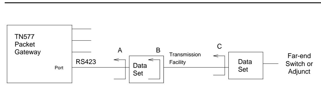
Figure 9-75. Packet Gateway Port Remote Loop-Around Test
