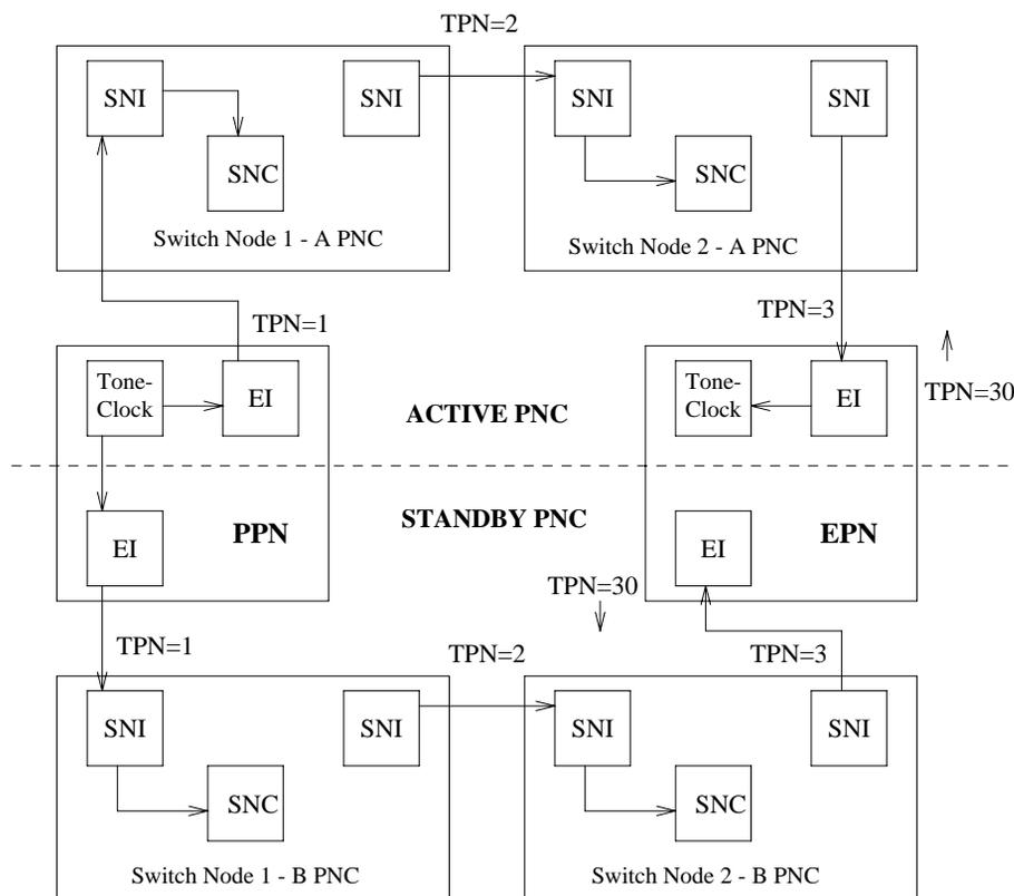
Timing information is sent through both the active and standby PNCs, but the EPNs normally derive timing from the EIs on the active PNC.
