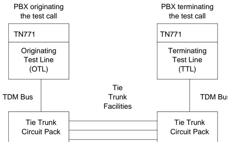
Figure 9-63. ATMS Tie Trunk Test Call
