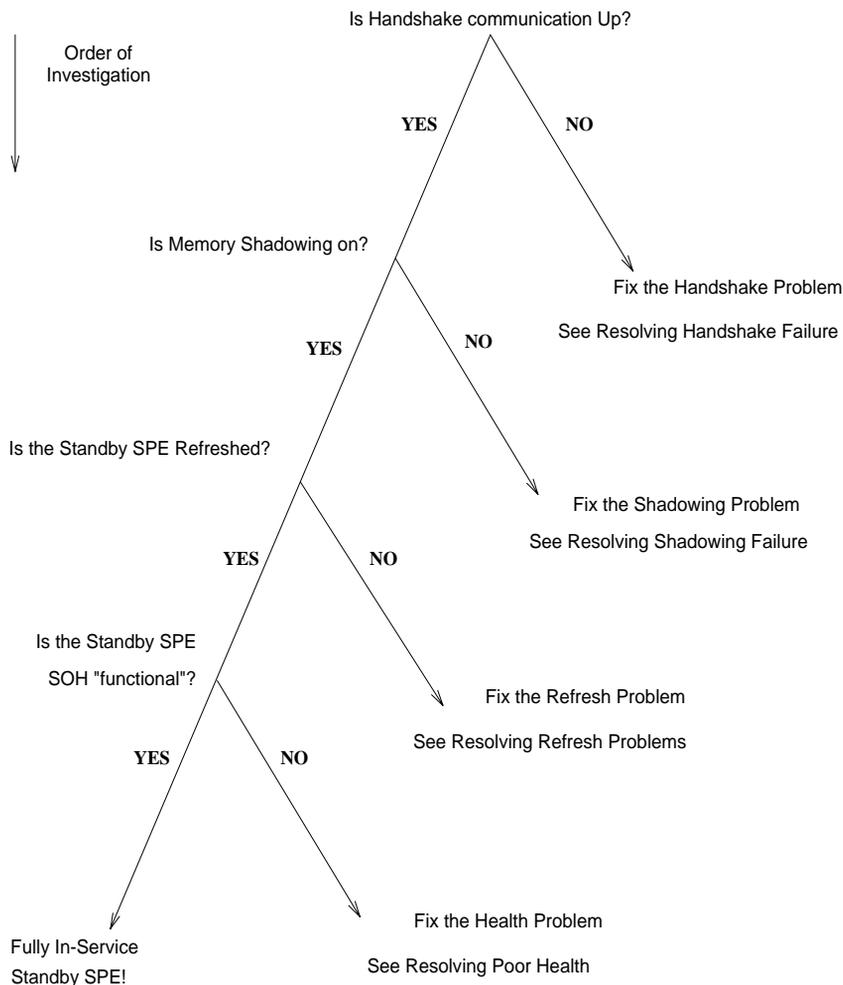
Figure 9-92. Resolving Standby-SPE Errors
