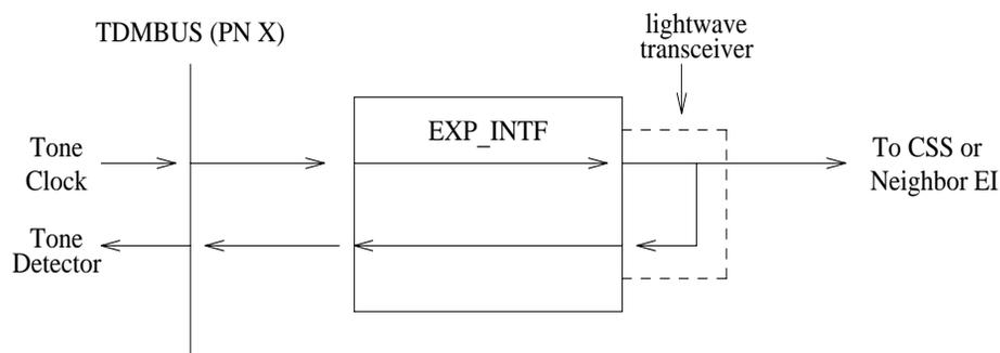
Figure 9-42. TDM BUS Lightwave Transceiver Looparound
