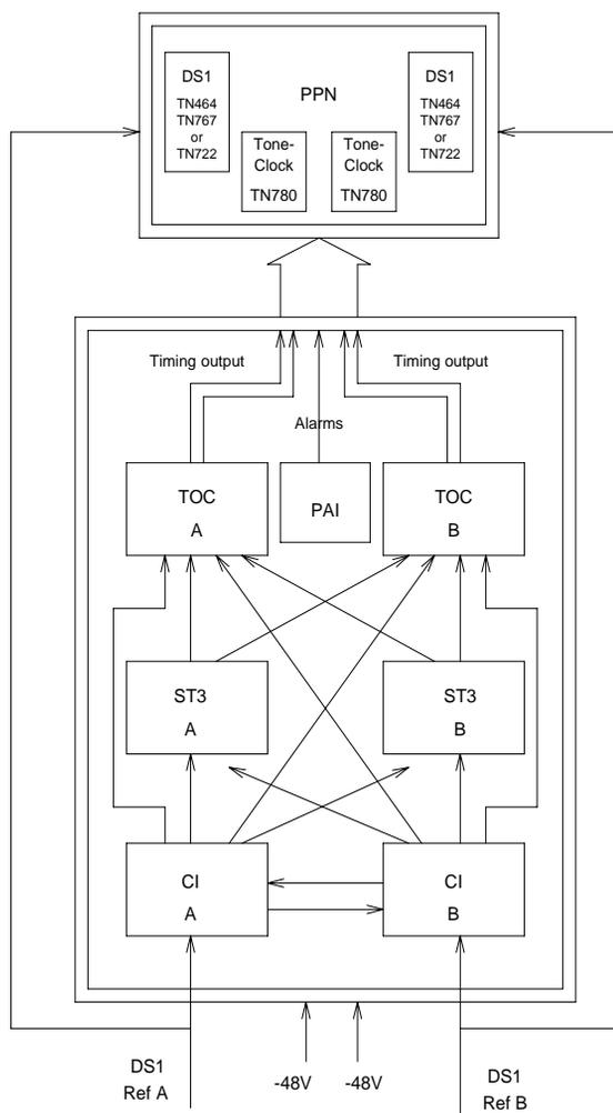
**Figure 9-93. Stratum 3 Clock Hardware Configuration**
