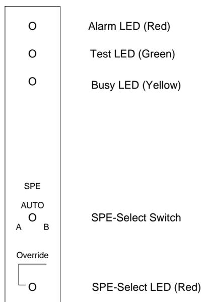
Figure 7-2. Duplication Interface Circuit Pack LEDs
