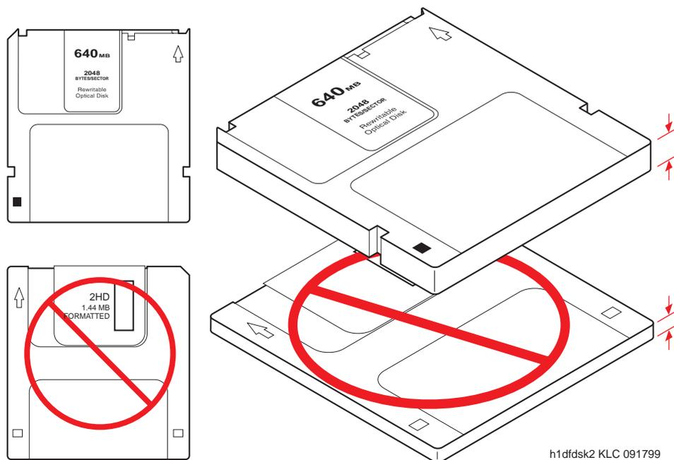
Figure 9-82. Use a 640Mb optical disk only, not a 1.44Mb floppy disk
