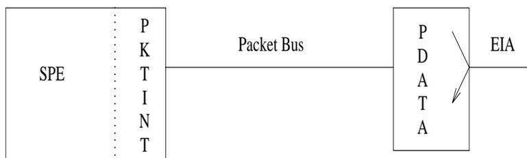
Figure 9-68. Configuration for LAPD Connectivity Test
