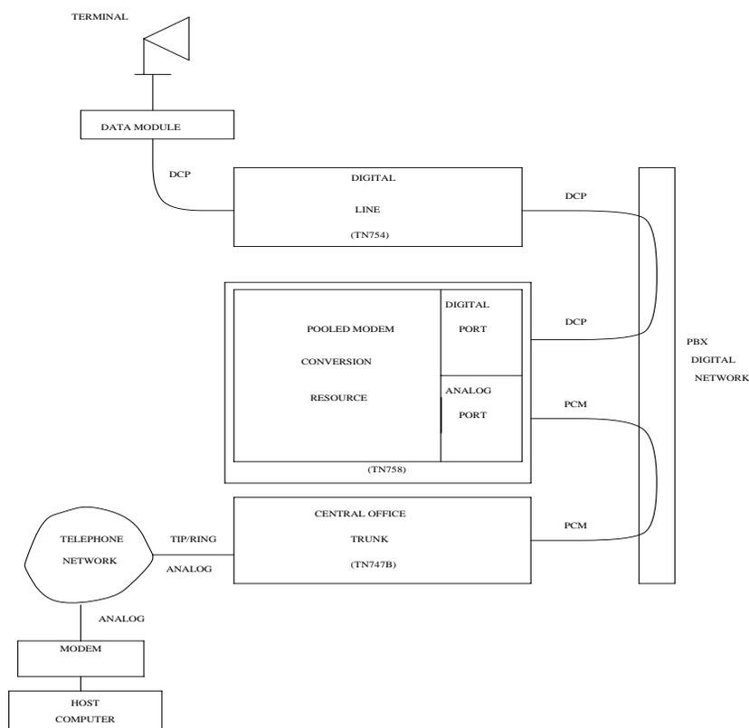
**Figure 9-60. Typical Modem Pool Switched Connection with Integrated Pooled Modem**
