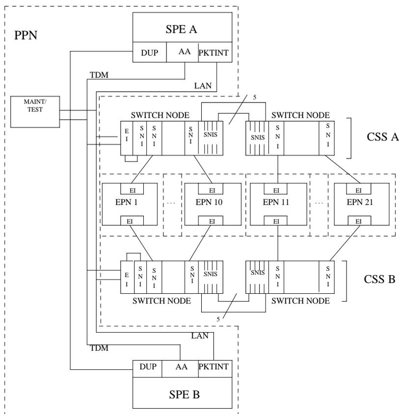
Figure 9-79. Duplicated PNC with Center Stage Switch
