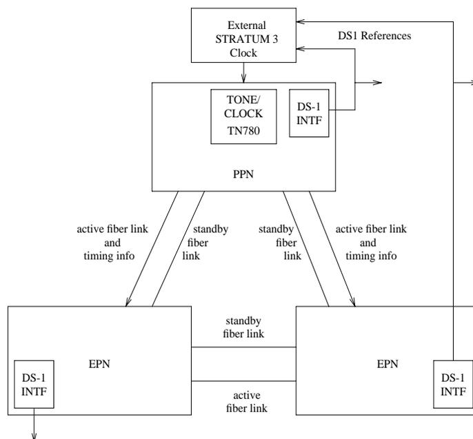
\* The EPN to EPN fiber link does not carry timing
