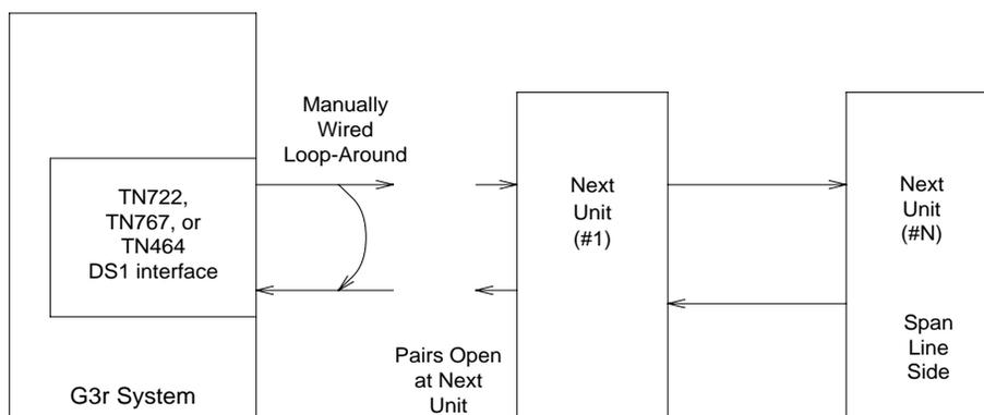
**Figure 9-103. Manual Looparound for Facility Fault Sectionalization**
