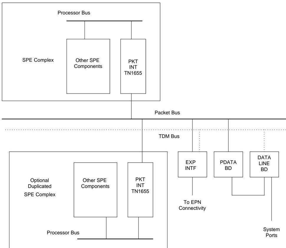
Figure 9-77. Packet Interface Connectivity
