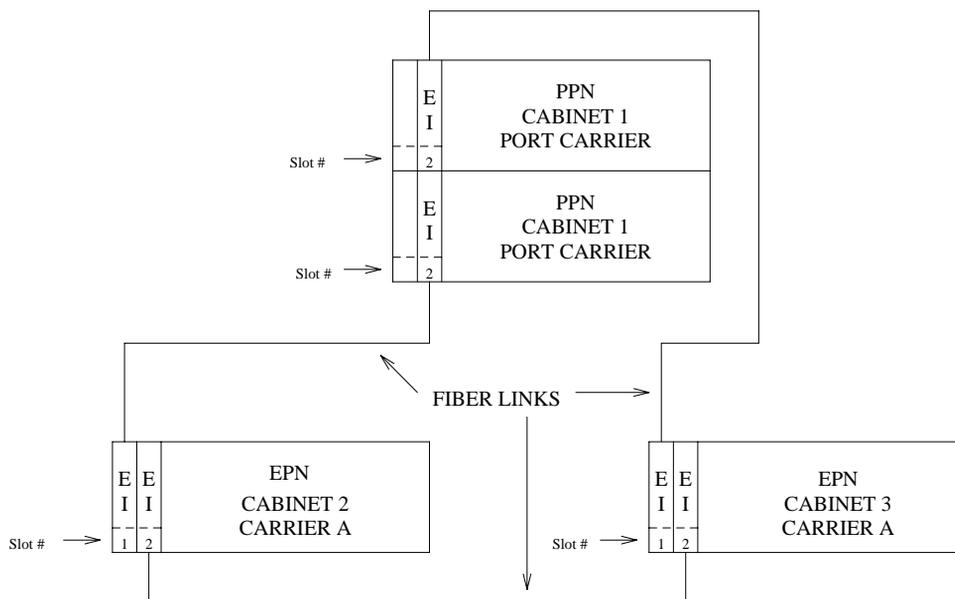
**Figure 9-35. Direct Connect Configuration with Simplex PNC**
