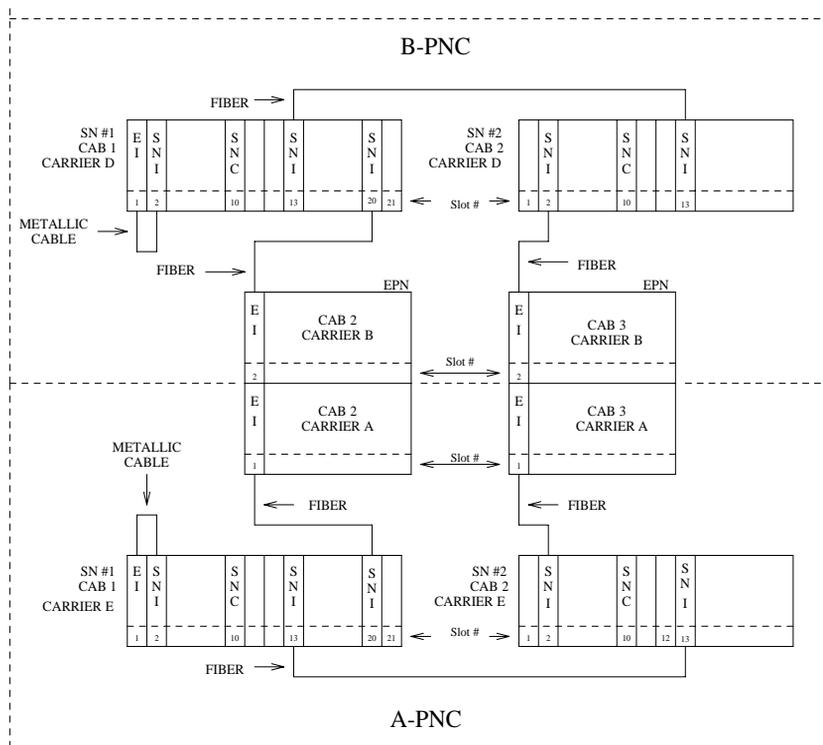
**Figure 9-38. Center Stage Switch Configuration with Duplicated PNC**
