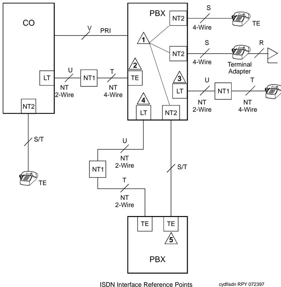
Figure 9-109. Integrated Trunk-Side BRI, ISDN Interface Reference points
