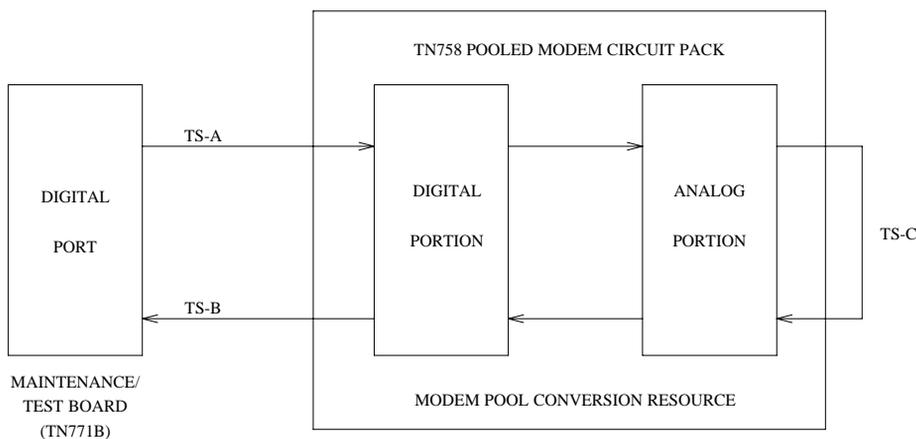
Figure 9-62. Modem Pool Conversion Resource Loop-Around
