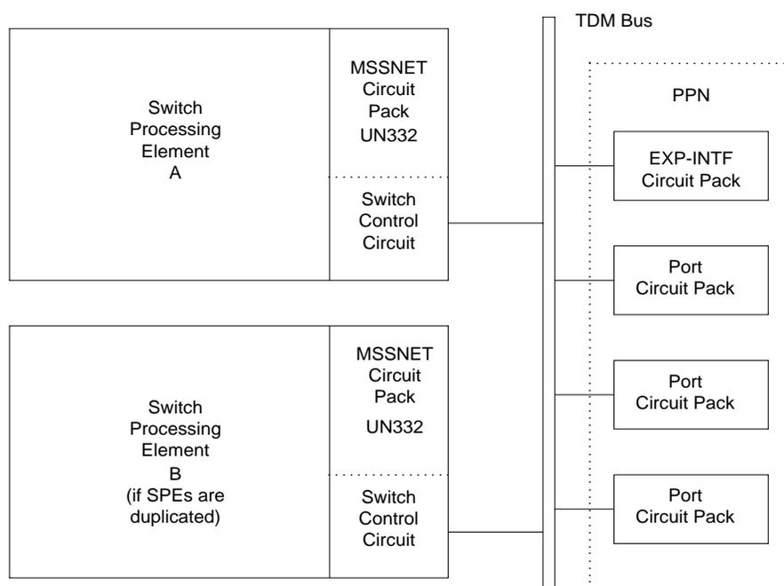
Figure 9-94. Switch Control Connectivity
