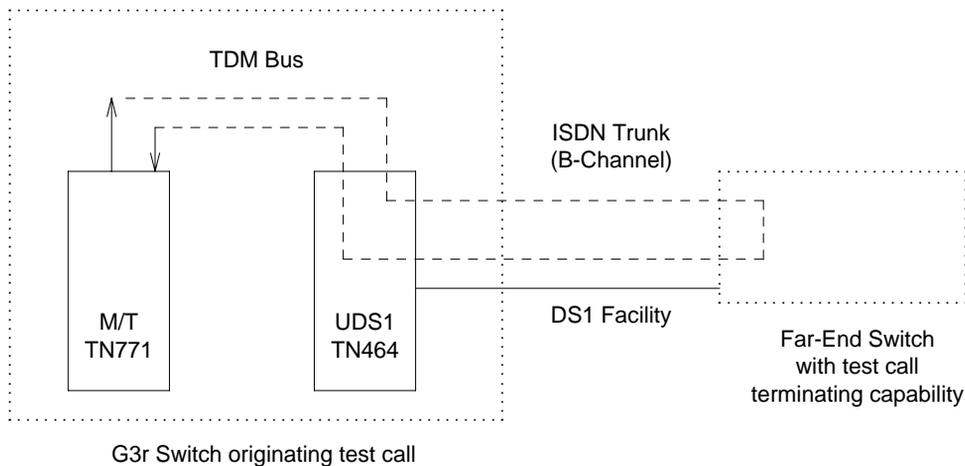
Figure 9-51. Outgoing ISDN-PRI Test Call
