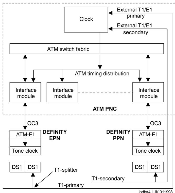
Figure 9-10. Stratum 4 synchronization with simple ATM PNC
