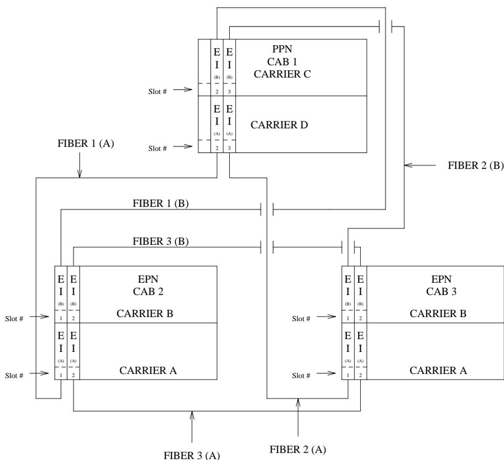
**Figure 9-36. Direct Connect Configuration with Duplicated PNC**
