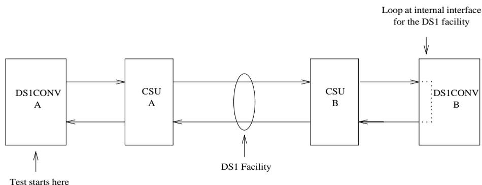
Figure 9-28. Far-End Internal Loopback Test (#797)
