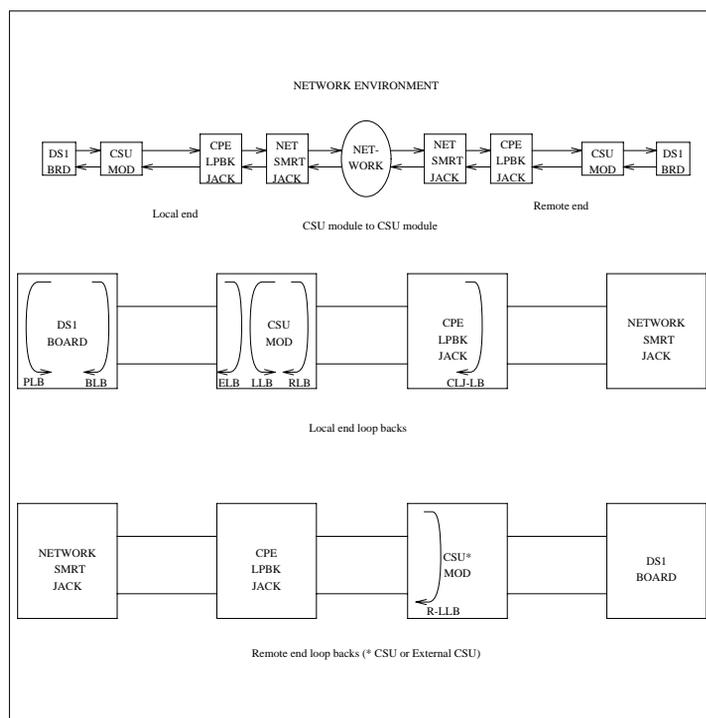
Figure 9-24. High Level Overview Of Loopback Points
