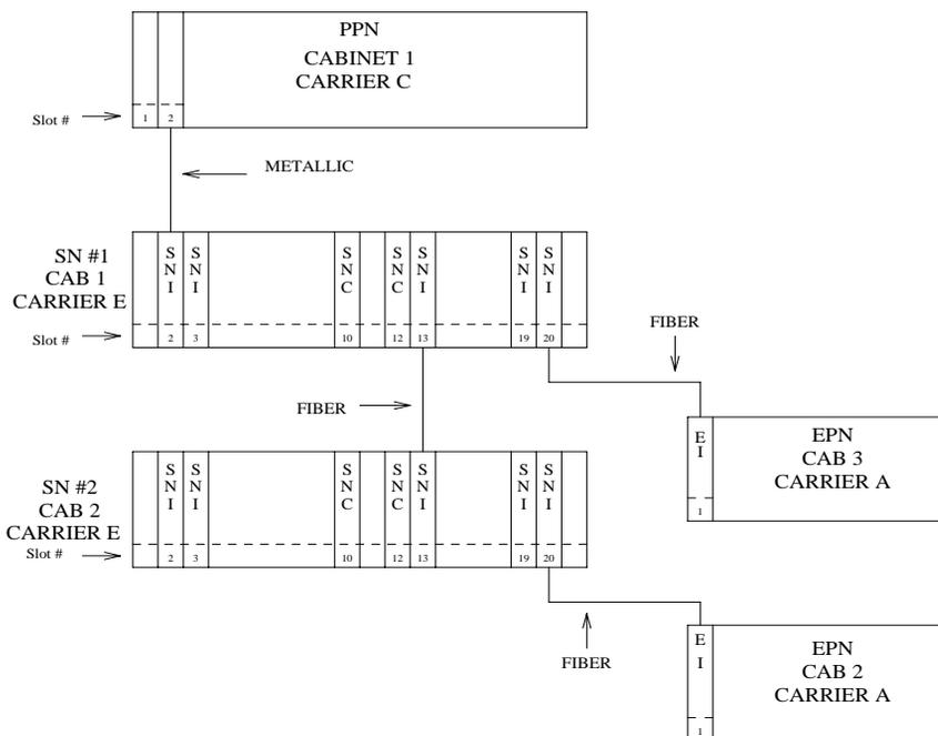
**Figure 9-37. Center Stage Switch Configuration with Simplex PNC**
