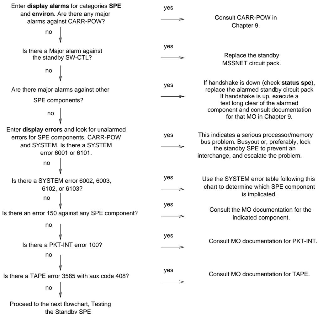
Figure 5-2. Determining the Cause of an SPE Interchange
