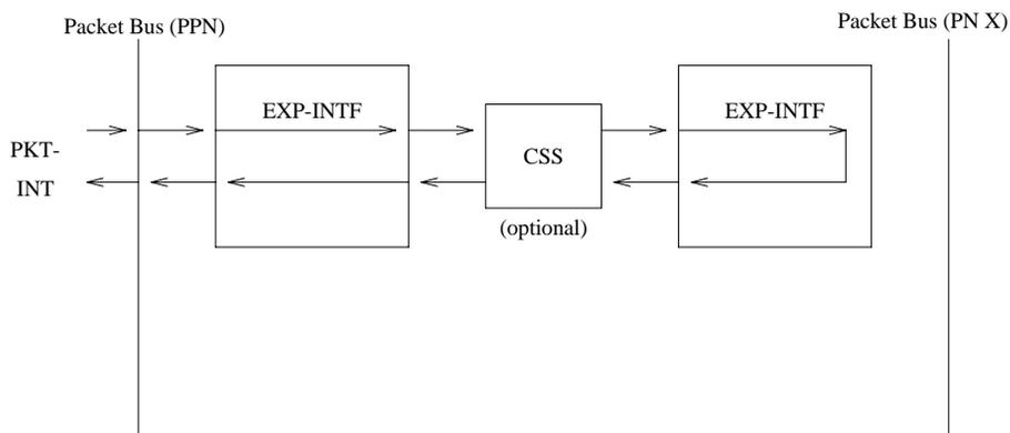
**Figure 9-46. Expansion Interface Packet Interface Test—PPN to EPN loop**
