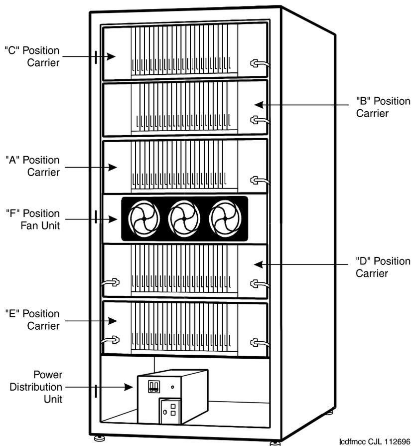
**Figure 9-22. Typical Multi-Carrier Cabinet with 649A Power Units**
