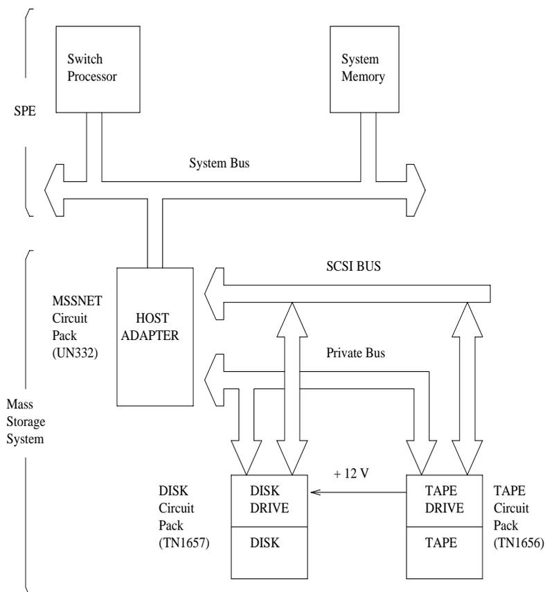
Figure 9-105. Mass Storage System Interactions
