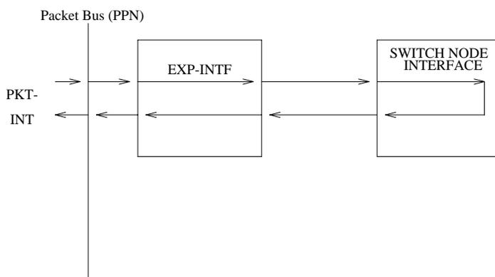
**Figure 9-47. Expansion Interface Packet Interface Test—PPN to CSS Loop**
