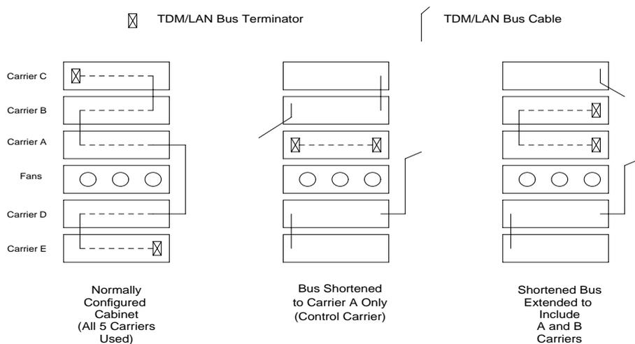
**Figure 5-47. Carrier Rewiring Example—Rear View of Multicarrier Cabinet**
