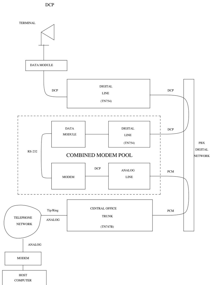
**Figure 9-61. Typical Modem Pool Switched Connection with Combined Modem Pool**
